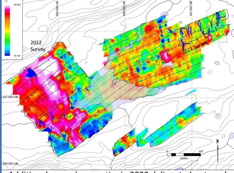
Additional ground magnetics in 2022 delineated a strongly magnetic body extending across the valley over a 1.4 km strike, open to north and south.
